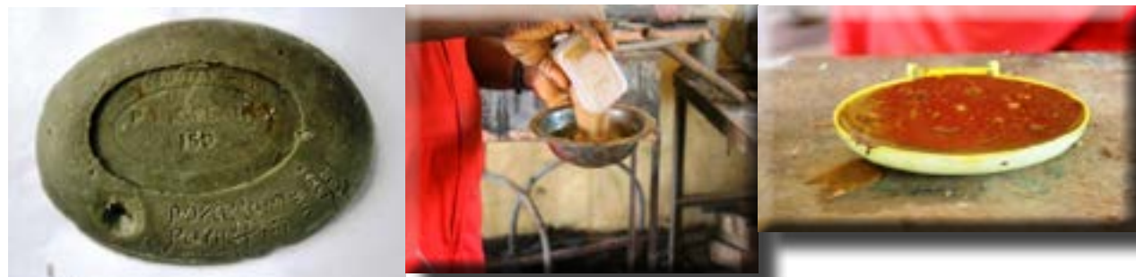
Plate 9: mixing and blending the ceramic sanitary grits with melted beeswax
