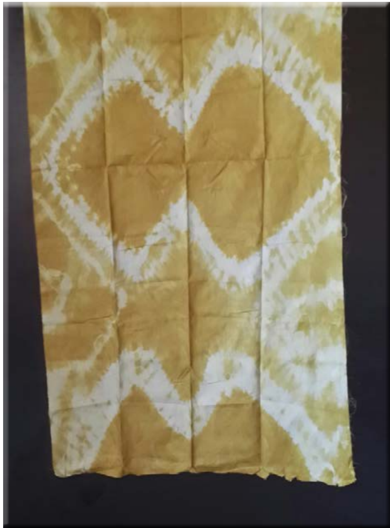
Plate 9: Resultant Dyed Fabric from an Aqueous Solution of Allium Cepa Mordanted with Solid Mass of Alum. Photo: Paul Aikhionbare, 2018
