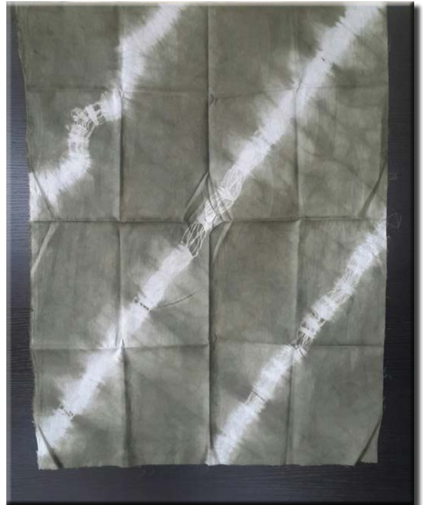
Plate 17: Resultant Dyed Fabric from the Alcoholic Dye Extract of Allium Cepa using Ferrous Sulphate Mordant. Photo: Paul Aikhionbare, 2019
