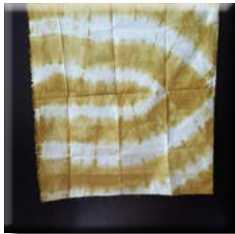
Plate 10: Resultant Dyed Fabric from an Aqueous Solution of Allium Cepa Mordanted with 100g of Alum. Photo: Paul Aikhionbare, 2018
