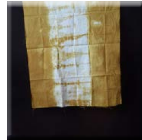
Plate 11: Resultant Dyed Fabric from an Aqueous Solution of Allium Cepa Mordanted with 250g of Alum. Photo: Paul Aikhionbare, 2018
